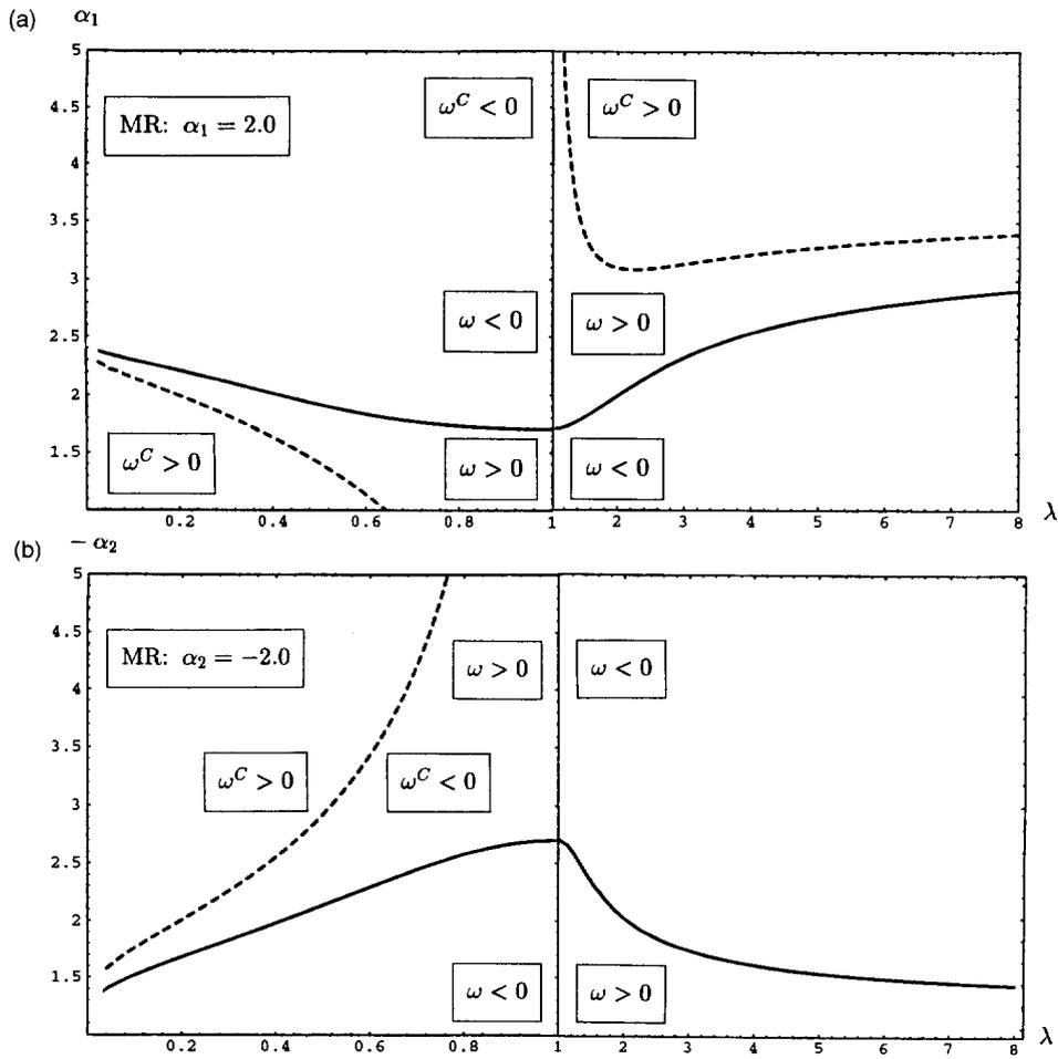
Fig. 7. Four-parameter model: functions  $\omega = 0$  and  $\omega_c = 0$  dependent on (a) material parameter  $\alpha_1$  and  $\lambda$ , (b) material parameter  $-\alpha_2$  and  $\lambda$ .
