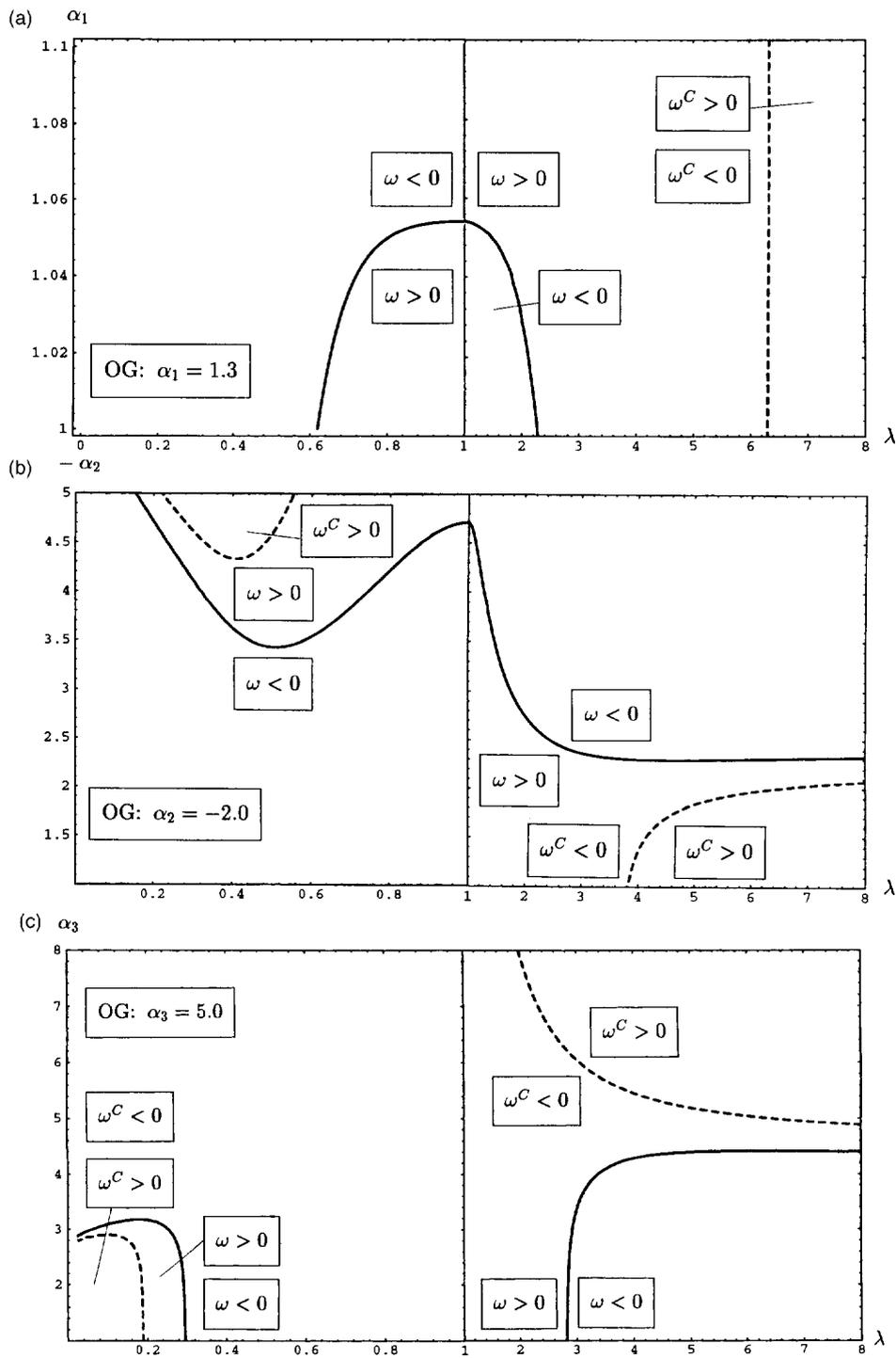
Fig. 5. Six-parameter model: functions  $\omega = 0$  and  $\omega_c = 0$  dependent on (a) material parameter  $\alpha_1$  and  $\lambda$ , (b) material parameter  $-\alpha_2$  and  $\lambda$ , (c) material parameter  $\alpha_3$  and  $\lambda$ .
