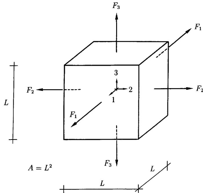
Fig. 1. Cube under triaxial tension.
