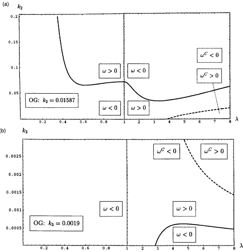
Fig. 6. Six-parameter model: functions  $\omega = 0$  and  $\omega^C = 0$  dependent on (a) material parameter  $k_2$  and  $-\mu_2/\mu_1$  and  $\lambda$ , (b) material parameter ratio  $k_3 = -\mu_3/\mu_1$  and  $\lambda$ .
